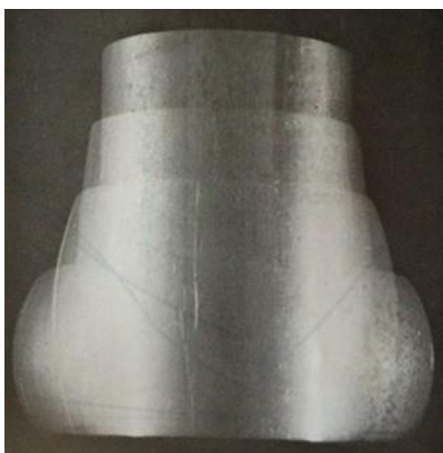
Fig. 2 Barreling in compressing a round solid cylindrical specimen between flat dies.
