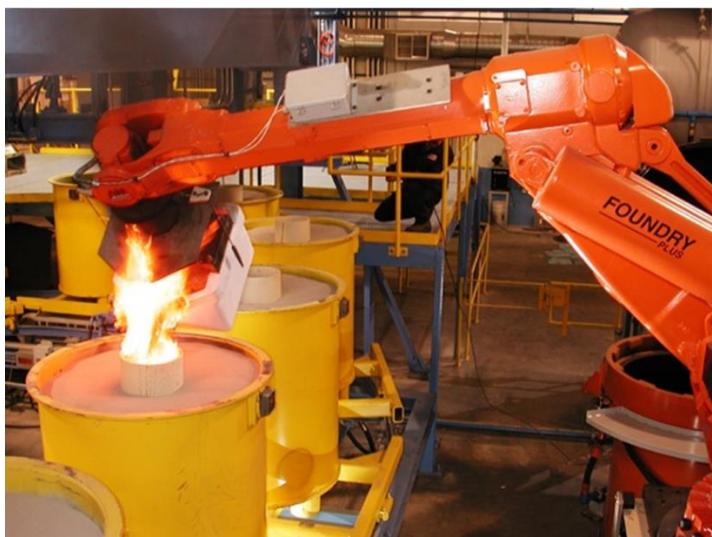
Fig. 5 (a) Metal is poured into mold for lost foam casting of a 60 hp, three-cylinder marine engine, (b) finished engine block.
