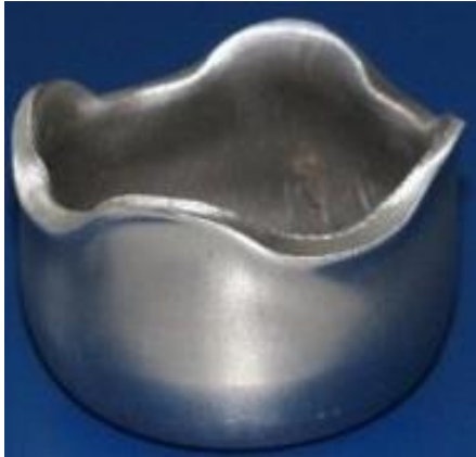
Fig. 5 Earing in a drawn cup, caused by the planar anisotropy of the sheet metal.
