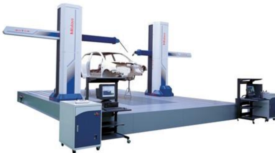
Fig. 2 A large coordinate-measuring machine with two heads measuring various dimensions on a car body.
