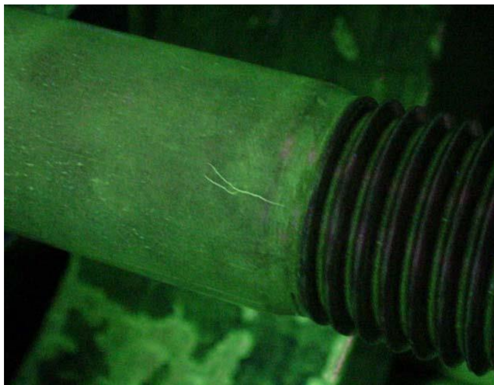
Fluorescent, Wet Particle Method
