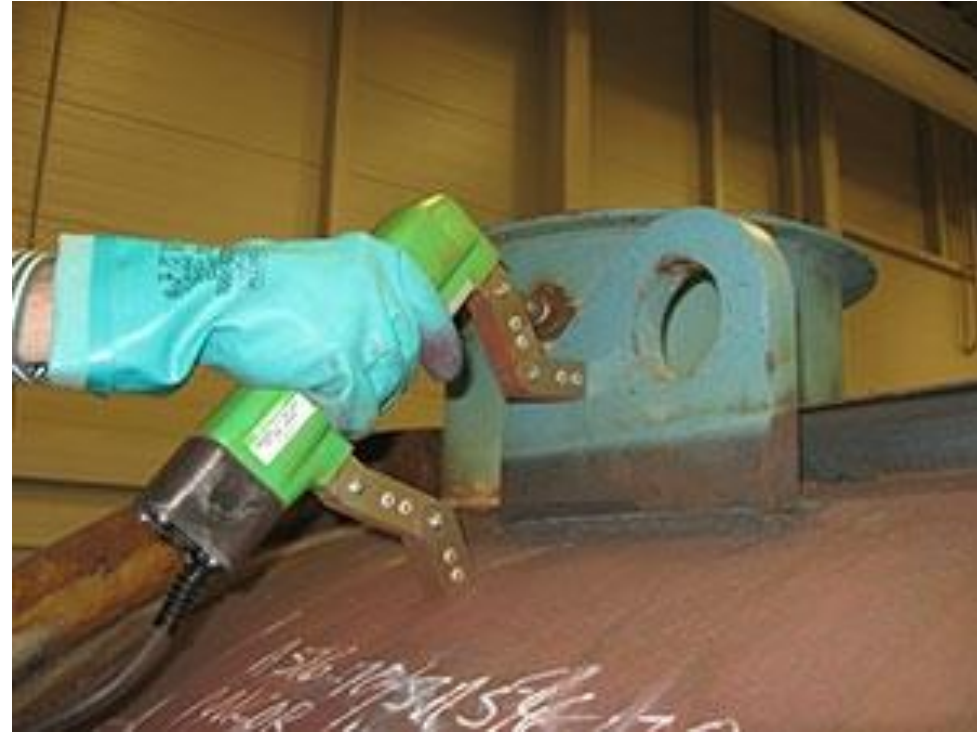
MT examination of a lifting lug weld on an inservice boiler.
