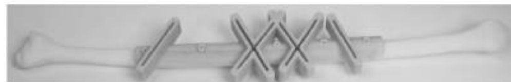
ULTEM 9085 FDM process: fibula guide placed on PolyJet model of fibula bone.
