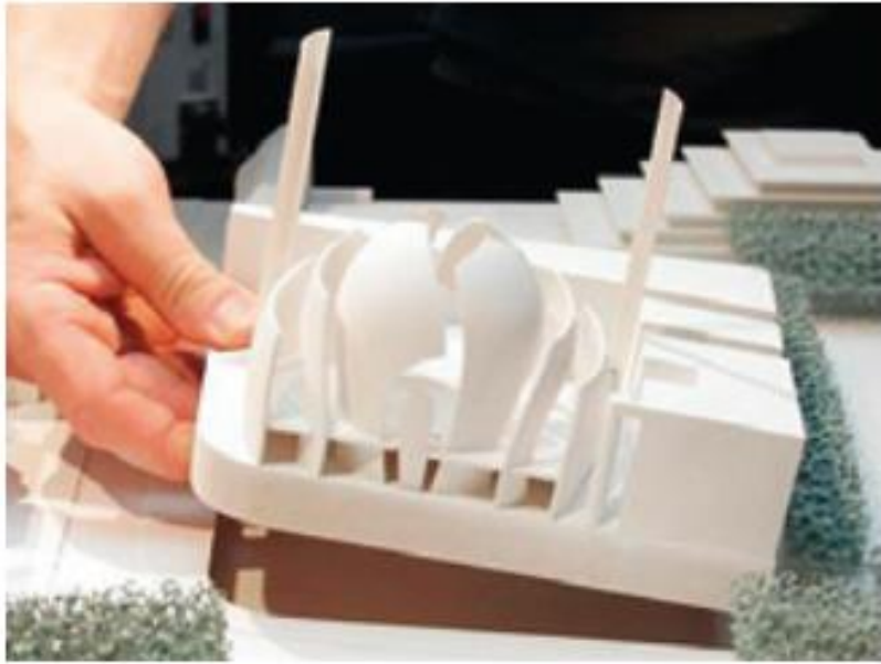
FIGURE 3.37 Architectural model, mosque, laser sintering (Source: Deutschlandwoche, 10/2007)
