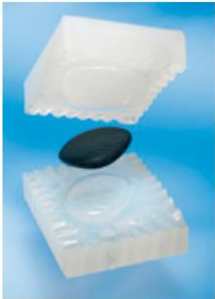
FIGURE 3.7 Speakers, stereolithography master and silicon mold (left), cast part (RTV, right) (Source: CP-GmbH)
