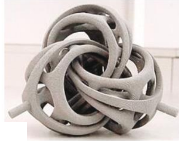
RE 3.23 Art objects; metal 3D printing (Prometal); part after AM production (left) and after post-processing and finishing by surface treatment (Source: Prometal, Bathsheba)
