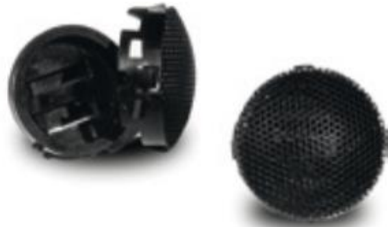
FIGURE 3.7 Speakers, stereolithography master and silicon mold (left), cast part (RTV, right) (Source: CP-GmbH)
