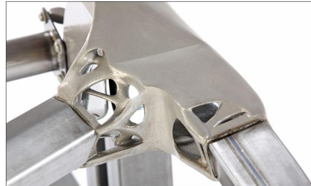
Fig. 3 In the NextGen spaceframe concept the AM nodes are part of an adaptable and flexible production concept that can produce vehicle structures 'just in sequence' (JIS), tailored for different load stages
