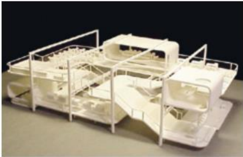
FIGURE 3.38 3D display of a concept for a touristic center, laser sintering of polyamides (Source: Bernhard Bader)
