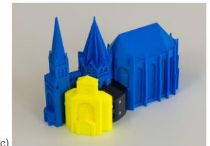
Figure 4.50 Model of the Aachen cathedral, fused deposition modeling. The CAD data were reconstructed from images and processed for model building: (a) full model, scale around 1 : 468, (b) detail of the roof, with deliberate extrusion structure, (c) important parts of the building history produced as single parts (Source: FH Aachen/Einhard Gymnasium Aachen)
