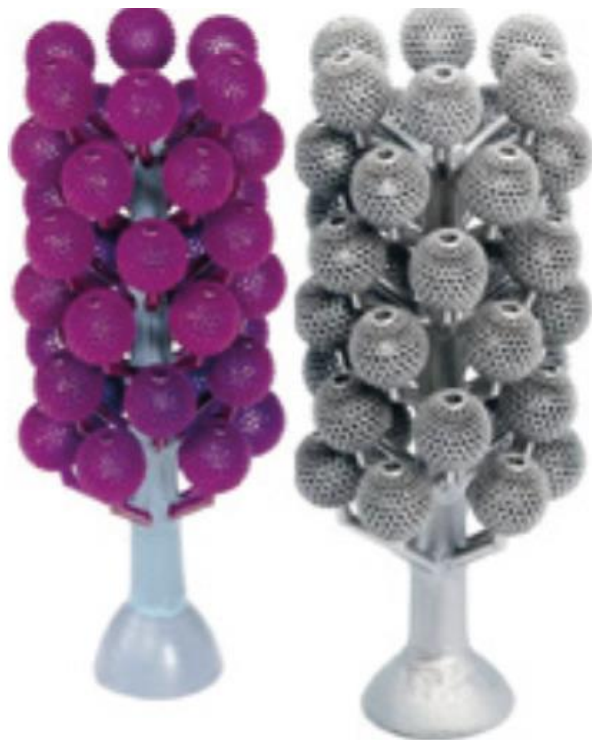
Fig. 14.11 Rings for investment casting, made using a ProJet ® CPX 3D Printer (Courtesy 3D Systems)
