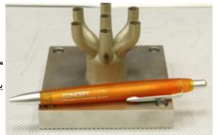
Fig. 4 The first test piece produced on the M2 cusing machine (Courtesy NASA/MSFC/Andy Hardin)
