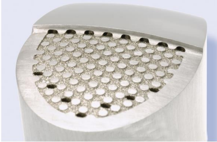
Figure 5.26 LaserCUSING, mold insert with conformal cooling, sliced part (Source: Concept Laser)
