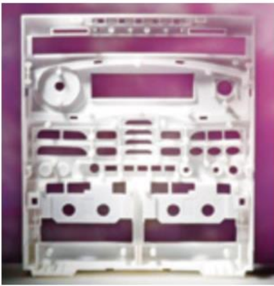
FIGURE 3.6 Dashboard insert; laser sintering, polyamide (left); fuel tank. laser sintering polyamide (right). both: 1 : 1 scale (Source: EOS)
