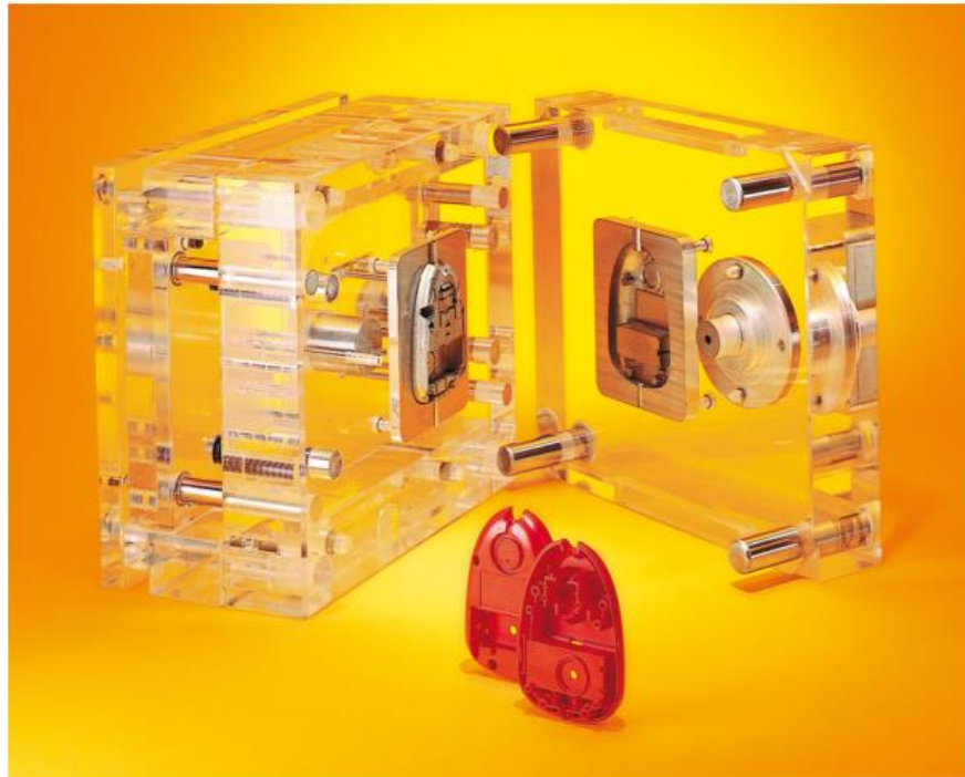
Figure 5.5 Basic setup of an injection mold with plates made of Plexiglas for demonstra purposes (Source: 3D Systems)
