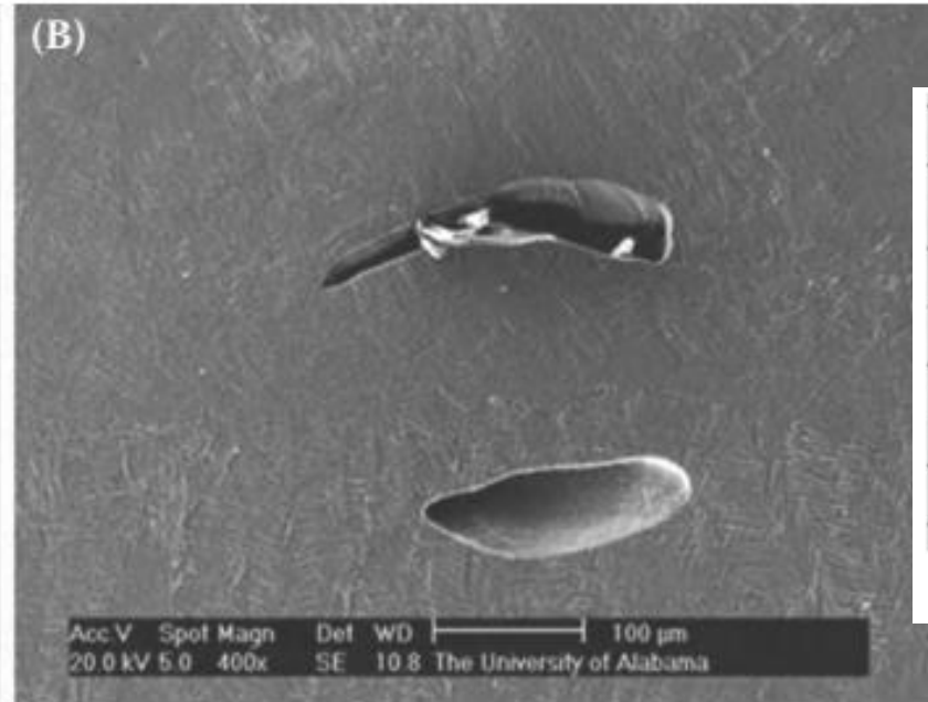
FIGURE 7.21 SEM micrograph showing porosity and unmelted powder in SF 65 sample: (A) unmelted powder, and (B) pores.
