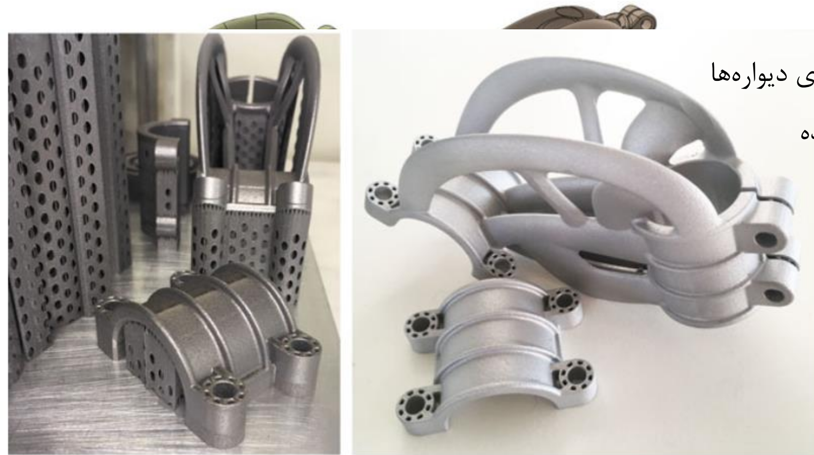
Fig. 9.34 Printed parts still attached to build platform with supports, and parts after post-processing and shot-peening
