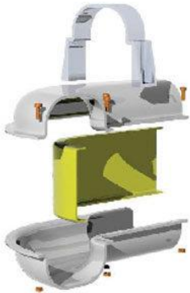
Duct: conventional Assembled, vacuum form Part Count = 16 plus glue
