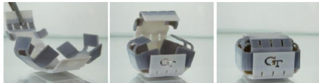
4D-printed unfolded box composed of shape memory polymers
