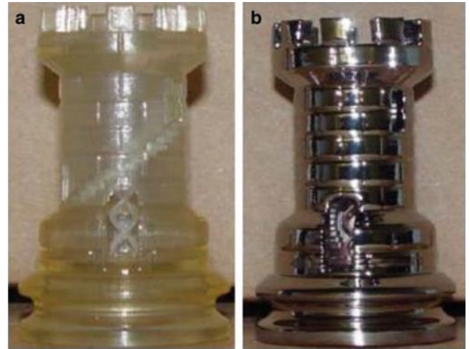
Fig. 16.6 Stereolithography part (a) before and (b) after chrome plating. (photo courtesy of Artcraft Plating)
