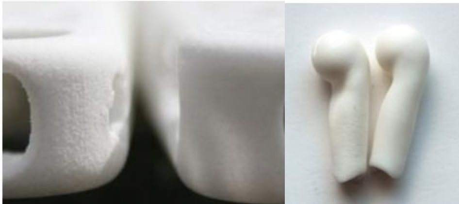
Examples of tumbled AM parts,
