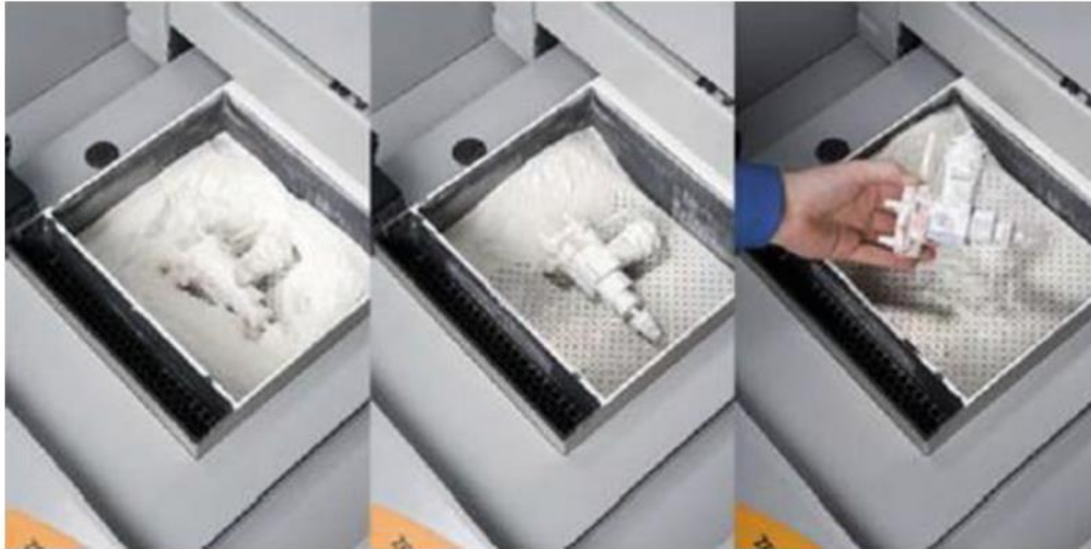
Fig. 16.1 Automated powder removal using vibratory and vacuum assist in a Z Corp 450 machine. (Photo courtesy of Z Corporation)
