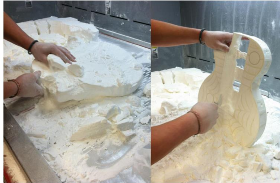
Fig. 12.6 Powder bed fusion parts being removed from the powder 'cake'
